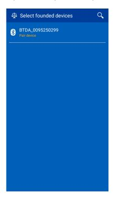
When they have been paired, the instrument's model and firmware are displayed. Tap again to start remotely controlling the scale.
